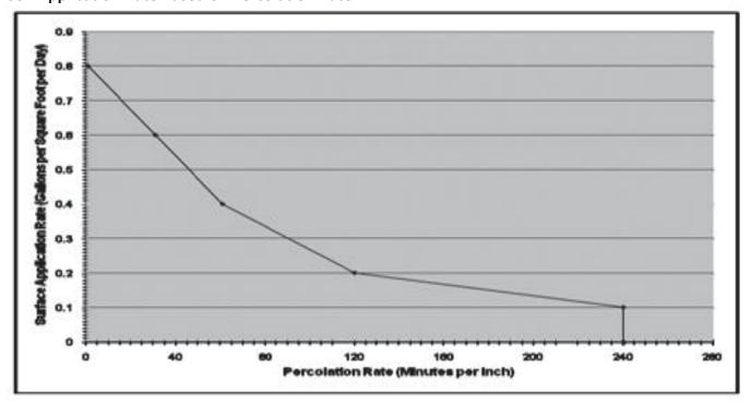
Soil application rates derived from percolation test results shall be calculated by using the slowest percolation test result obtained from all percolation soil profile borings in the area in which the disposal field will be located.
